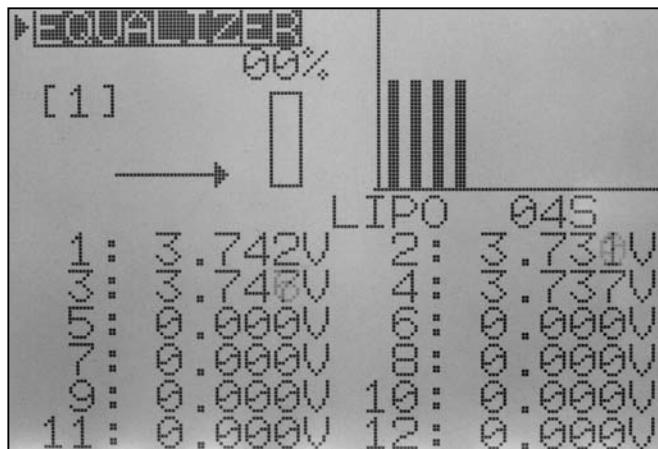
**For accurate cell voltage measurement it is essential to connect the battery charge lead (positive and negative) to the unit in addition to the voltage sensor lead, in order to obtain the same potential for each cell.**
