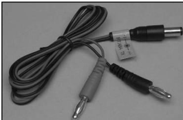
Transmitter battery charge lead
