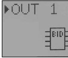
If a BID chip is connected, a BID symbol appears in the "OUT 1 Data" menu, and the list of battery settings is expanded.
