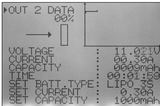
The battery parameters are defined using the three set-up points battery type, charge current and capacity.
