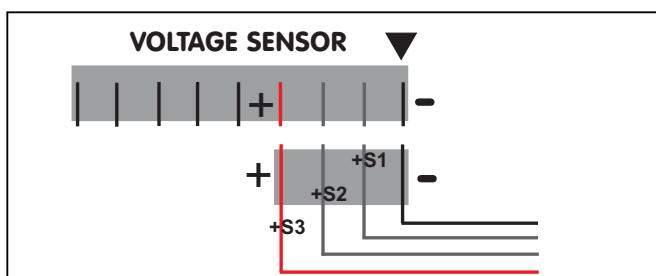
Diagram of the voltage sensor lead pin-outs.
