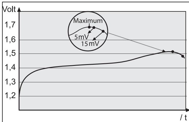
The graph above shows the typical charge curve of an NC or NiMH battery. At the end of the charge process the pack's internal resistance changes as the cells heat up.
