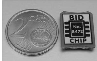
BID chip without lead, for fitting to batteries
