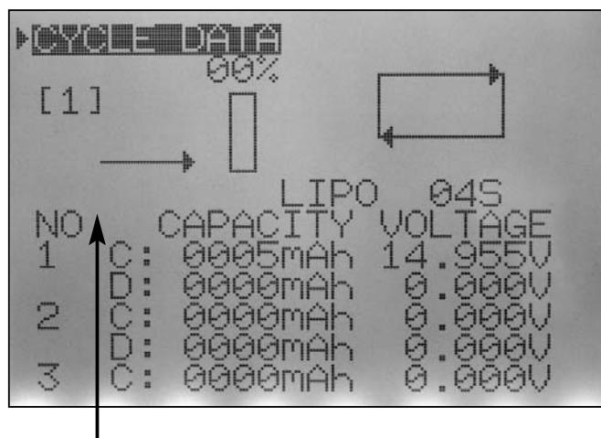
On-screen display of the current cycle. In this example Cycle 1 of two pre-selected cycles is currently in progress.
