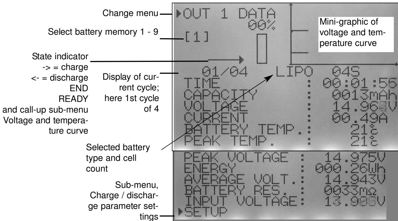
The charger features nine internal battery memories [1] ... [9] in which you can store settings for the charge and discharge parameters. The nine battery memories can be configured in any way you wish.
