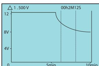
can display the battery voltage in curve form. To see this, move the cursor to the second line and press Enter; pressing Enter again closes the window.
