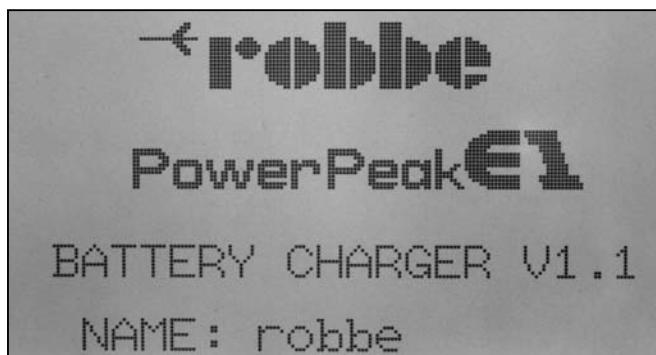
Wait for the charger to conclude its self-calibration process (LEDs go out), then press the Enter button: the display for the OUT 1 output appears on the screen.
